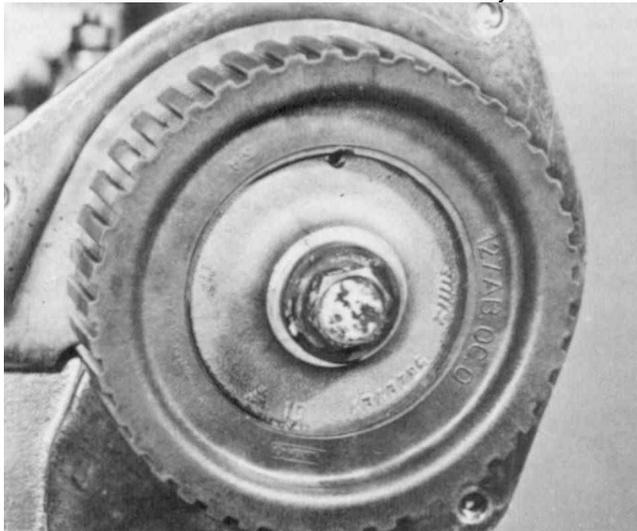
3.56 Fit the camshaft toothed pulley
