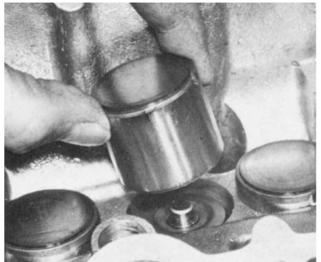
3.49D Refit each tappet bucket with its shim to its valve
