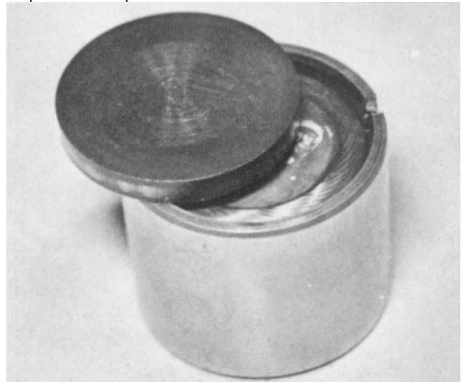
3.49B ...prise out the valve clearance adjusting shim
