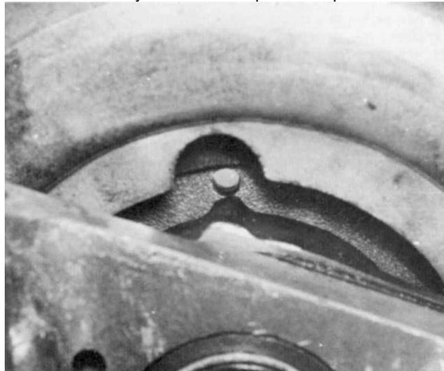
3.59 Hole in pulley aligned with část ridge, view from behind the wheel
