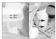
The coolant expansion tank is located in one of two places (see *Underbonnet check points* on pages 0•10 and 0•11). The coolant level can vary with engine temperature. When cold, it should be between the MAX and MIN marks. When the engine is hot, the level may rise slightly above the MAX mark.
