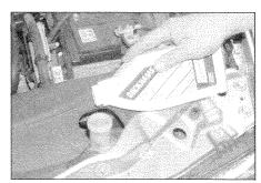
Add a mixture of water and antifreeze to the expansion tank until the coolant level is halfway between the level marks. Refit the cap and tighten it securely.
