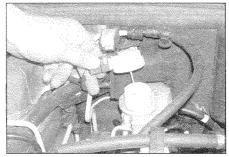
2 If topping-up is necessary, modernic the area around the filler cap to prevent dirt entering the hydraulic system. Unscrew the reservoir cap and carefully lift it out of position, holding the wiring connector plug and taking care not to damage the level sender float. Inspect the reservoir; if the fluid is dirty, the hydraulic system should be bled through (see Chapter 1).
