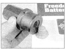
3 If corrosion (white, fluffy deposits) is evident, remove the cables from the battery terminals, clean them with a small wire brush, then refit them. Automotive stores sell a tool for cleaning the battery post . . .
