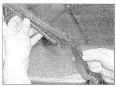
3 Don't forget to check the rear wiper blade as well. To remove the blade, press in the catch at the base of the arm, and slide the blade and upper section of the arm out.
