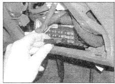
3 To replace a blown fuse, simply pull it out using the plastic tweezers provided. Fit a new fuse of the same rating (see Chapter 12). If the fuse blows again, it is important that you find out why - a complete checking procedure is given in Chapter 12.
