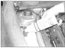
To top-up the level, pull the filter inside the filler neck upwards until it clicks - this can now be used as a funnel. When topping-up the reservoir, a screenwash additive should be added in the quantities recommended on the bottle.
