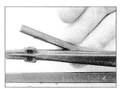
1 Check the condition of the wiper blades; if they are cracked or show any signs of deterioration, or if the glass swept area is smeared, renew them. Wiper blades should be renewed annually.
