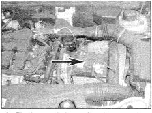
The battery is located at the front of the engine compartment on the left-hand side. The exterior of the battery should be inspected periodically for damage such as a cracked case or cover
