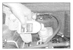
Carefully add fluid, taking care not to spill it onto the surrounding components. Use only the specified fluid; mixing different types can cause damage to the system. After topping-up to the correct level, securely refit the cap and wipe off any spilt fluid. Reconnect the fluid level wiring connector.
