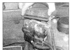
If more than one indicator light or headlight has failed, it is likely that either a fuse has blown or that there is a fault in the circuit (see Chapter 12). The main fuses are located in the fusebox situated to the right of the steering wheel. Additional fuses are located behind the glovebox, with several enginerelated fuses on the engine compartment bulkhead or next to the battery.
