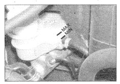
The MAX and MIN marks are indicated on the reservoir. The fluid level must be kept between the marks at all times
