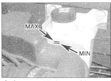
On most models, the reservoir is mounted at the rear of the engine, next to the brake fluid reservoir; 1.2 litre models have the reservoir by the engine (see Underbonnet check points on page 0.10). The fluid level can be viewed through the reservoir body, and should be between the MIN and MAX marks; if not, a dipstick is incorporated in the filler cap.
