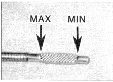
Note the oil level on the end of the dipstick, which should be in the hatched area between the upper (MAX) mark and lower (MIN) mark. Approximately 1.0 litre of oil will raise the level from the lower mark to the upper mark.
