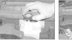
Start the engine and wait for the fluid level in the reservoir to stabilise before proceeding. With the engine running, turn the steering wheel fully left and right several times, returning to the straight-ahead position. Wait for the level to stabilise, then check the fluid level once more, and top-up if necessary. Switch off the engine on completion.
