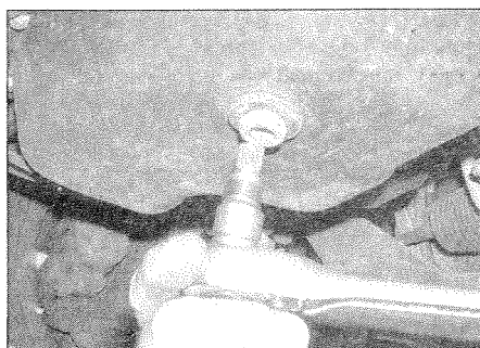
3.7 On some models, a special socket is required to loosen the sump drain plug
