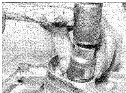
14.13b Using a socket to fit a new oil seal to the oil pump
