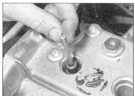
4.21c ... then insert the dowel rods
