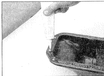
12.4 Applying sealant to the sump flange
