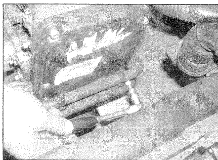
4.8a Unscrew the two mounting bracket bolts ...
