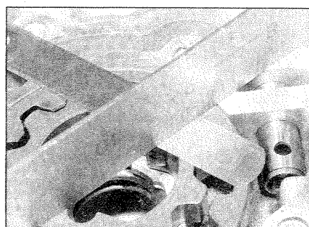
13.9b Measuring oil pump gear endfloat
