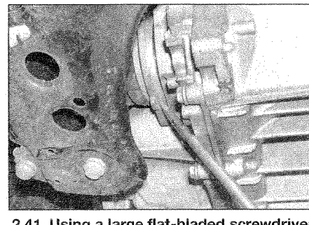
2.41 Using a large flat-bladed screwdriver to separate the driveshaft inner ends from the transmission
