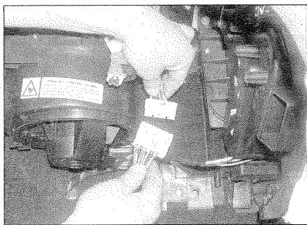
9.7 Disconnect the wiring near the heater motor
