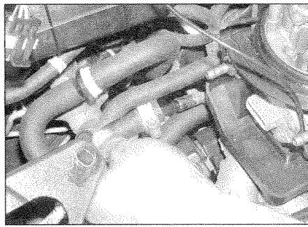
9.6 Unscrew the clip and disconnect the brake servo vacuum hose
