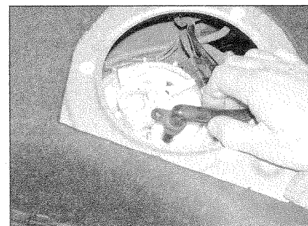
6.6 Disconnecting the fuel tank breather pipe
