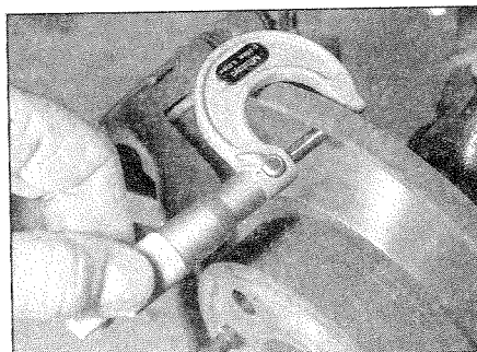
6.3 Measuring the brake disc thickness with a micrometer
