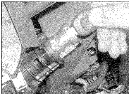
17.4b . . . and withdraw the lock and barrel from the housing
