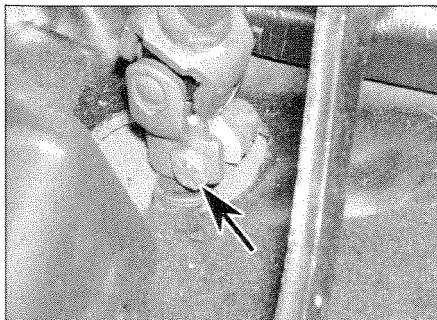
15.6 The clamp bolt attaching the steering column universal joint to the steering gear pinion shaft
