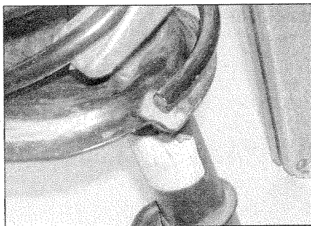
3.14 Make sure that the lower end of the coil spring is correctly located in the recess on the lower spring seat
