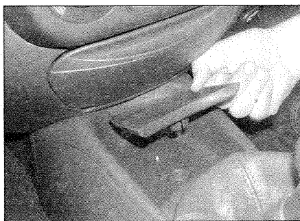
23.4a Remove the covering from the oddsments tray in the centre console ...
