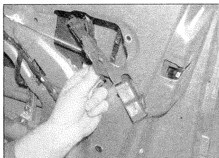
16.10 Removing the security cover from the front door lock operating rods
