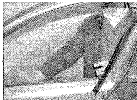
18.6 Tilt the front window glass forwards and remove it upwards
