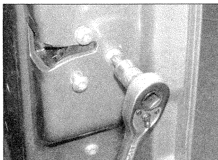
16.11 Removing the front door lock mounting screws
