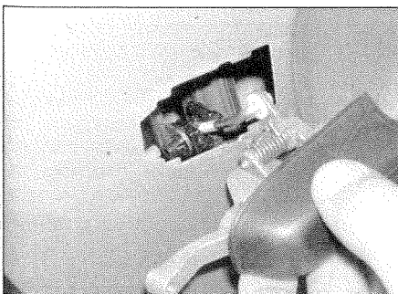
16.2e ... then swivel out the handle and release the plastic adjustment clip inside the door
