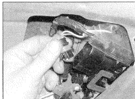
16.12c Disconnect the main wiring plug ...
