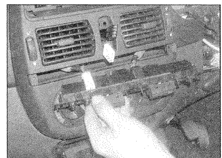
23.15b . . . and withdraw the switch panel from the front of the facia . . .
