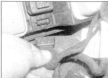
6.1 Disconnecting the wiring from the headlight unit
