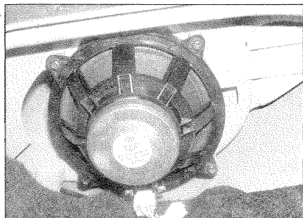
10.4 The rear loudspeaker viewed from the luggage compartment
