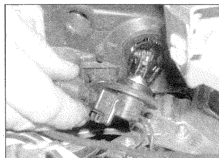
4.13 Twist the front direction indicator anticlockwise and remove it from the rear of the light unit ...
