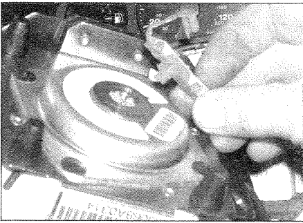
22.3b Disconnect the yellow wiring from the rear of the airbag
