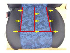
Once you've cut away 'ALL' the metal ring clips and removed them you can then fold over the cover. Those with heated seats, I have removed the heating elements and removed all the old wiring and connectors as shown.
