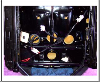
This is how I have currently set up my seats; if you prefer to use the wiring loom that came with the heating elements, just connect the orange and red wire to either of the red/green wires from the vehicles own wiring under the seat and the negative wire to either black wire under the seat.
