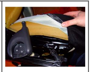
You may now have noticed that there are three metal rods running the whole length of the lower cushion and a strut rod near the front of the cushion (Shown as red lines). The yellow arrows point to metal ring clips that need to be removed. These ring clips hold the rods within the cover to a metal rod within the foam cushion. Whatever you do, do not cut the metal rods. Only the metal ring clips. Work your way left to right in a row removing the clips, try not to bend the metal rods in the cover.
