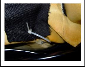
Reattach the cover to the sides of the seat, they basically fold over and push back in. You will hear them clip into place. Once complete feed the cover between the lower and upper cushion, make sure you don't trap any of the wiring and then reattach the clip to the bottom of the seats frame. This guide will explain how to reconfigure the wiring of the heated seats to work in the S, SX, HLX and HGT models. As with anything electrical disconnect the battery before attempting the wiring.
