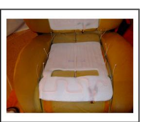
Carefully tilt the seat covering back over the cushion, pay attention to the front of the cushion so that it doesn't rise or move out of place. Make sure there are no folds or bends in the heater elements then start attaching the cable ties to the metal rods in the cover. Working left to right. Make sure the cover is stretched over properly and the strut rod sits in the crevice. Pull the cable ties tight, then cut off any excess, keep working your way back till all seven are done.
