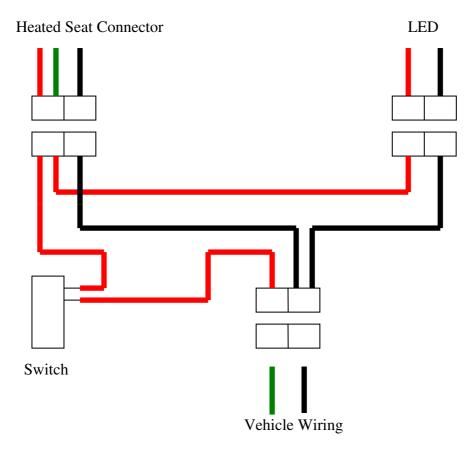
If you want to have permanent heat on the heated seats instead, then do not combine the red and the green wires together on the heated seat connector. Connect the red wire only. Tape up and insulate the green wire as it'll not be used.
