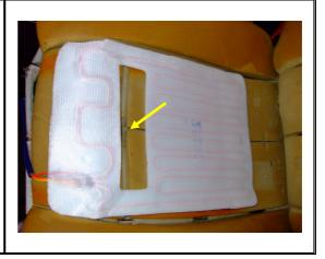
Once you are happy with the way the element is seated, get a screw driver and push a hole through the cushion directly where the wires exit the heating elements at an angle to the thinnest part of the foam cushion. Then use a sharp knife to make a 1.5cm gap then carefully feed the wiring through the hole. As can be seen in the photograph.
