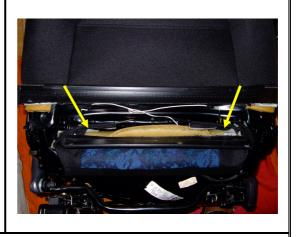
Now clip the two plastic clips from both ends of the cover (front and rear), so that they are perfectly reattached.
