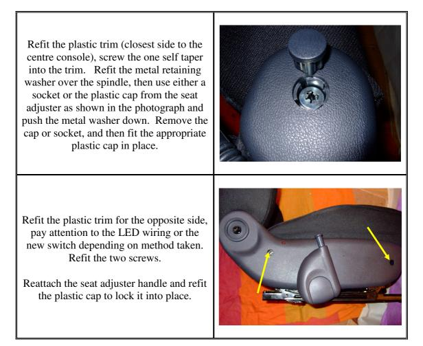
Refit the plastic surround to the seat; make sure the metal arm in the seat doesn't obstruct the surround. Carefully screw the two self tapers back into the surround and then carefully push the seat lever over the metal arm. Finish by refitting the screw into the lever and reconnecting the flap.
